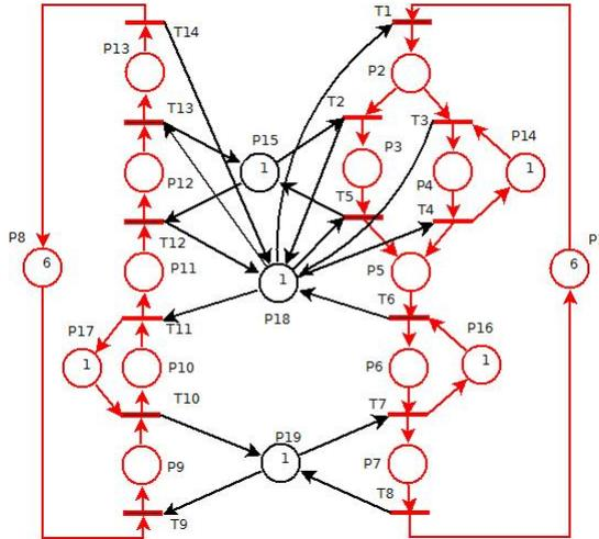
Fig. 4. PN3 model of a manufacturing system (after [9])
